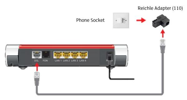
If your phone socket has a RJ-11 port, you can plug in the cable without using a Reichle adapter.
